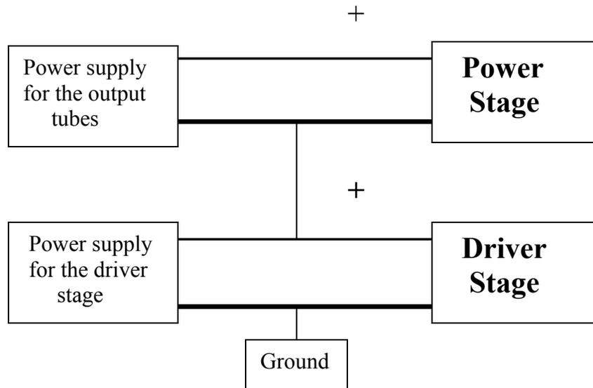
As you can see, only the negative line of the power supply of the drivers' stage is grounded, whereas the negative line of the Power supply of the output stages is not and it is connected to the positive line of the other power supply.
